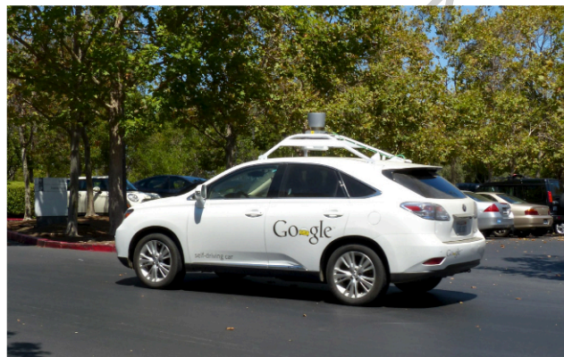
Figure 1.9 Google's Waymo, a self-driving car, can navigate roads, maintain safe speeds, and see obstacles in time to apply the brakes. (credit: "Google Self-Driving Car" by R Boed/Flickr, CC BY 2.0)
