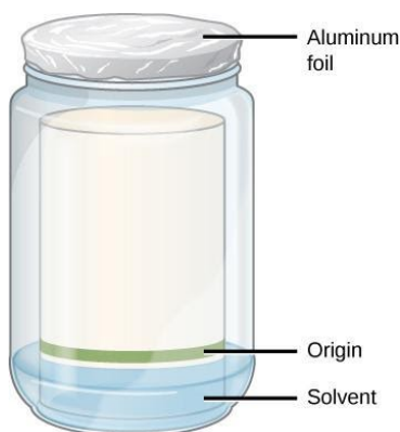
Figure 10.6: Chromatography can be set up in a container such as a Mason jar. The start line of the sample, the origin, is shown above the solvent.
