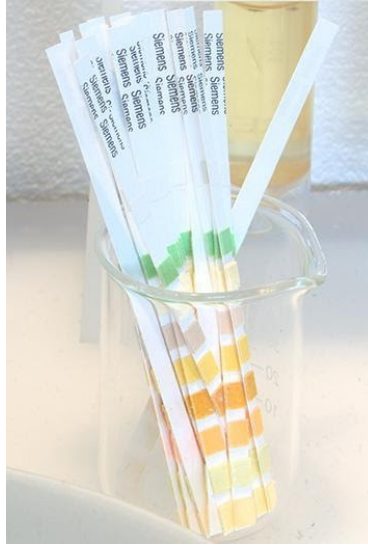
Figure 7.4: Diastix glucose detection strips turn from blue to green to yellow to brown with increasing concentrations of glucose.
