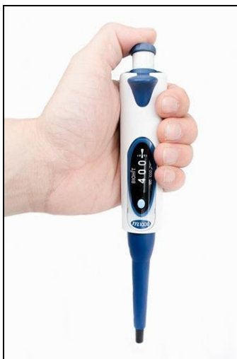
Figure 1.3: Micropipettes are used for measuring micro quantities of liquid from 1 to 1,000 \mu\text{l} .
