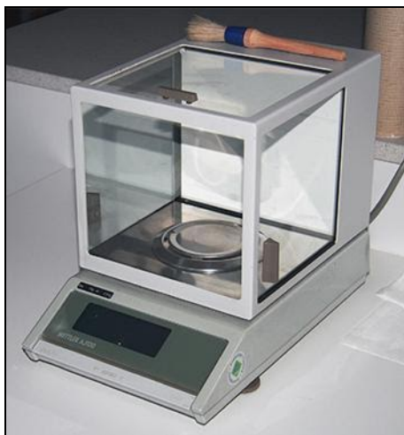
Figure 1.5: A scientific scale is used to find the mass of solids.
