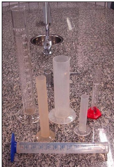
Figure 1.4: Graduated cylinders are used to measure volumes from 10 ml to 1 L.
