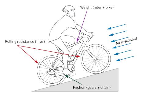
FIGURE 7.3 Several forces are at work when a person rides a bicycle. Understanding the physics of cycling does not guarantee that one knows how to ride a bicycle. (attribution: Copyright Rice University, OpenStax, under CC BY 4.0 license)
