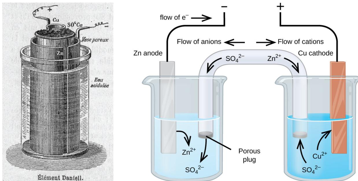
**FIGURE 17.8** Illustration of a Daniell cell taken from a 1904 journal publication (left) along with a simplified illustration depicting the electrochemistry of the cell (right). The 1904 design used a porous clay pot to both contain one of the half-cell's content and to serve as a salt bridge to the other half-cell.
