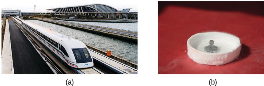
**FIGURE 19.11** (a) This magnetic levitation train (or maglev) uses superconductor technology to move along its tracks. (b) A magnet can be levitated using a dish like this as a superconductor. (credit a: modification of work by Alex Needham; credit b: modification of work by Kevin Jarrett)
