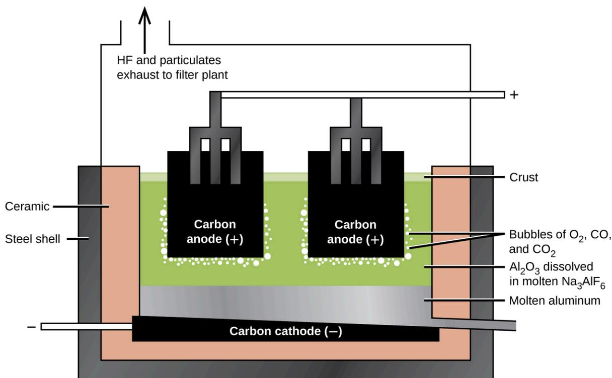
**FIGURE 18.11** An electrolytic cell is used for the production of aluminum. The electrolysis of a solution of cryolite and calcium fluoride results in aluminum metal at the cathode, and oxygen, carbon monoxide, and carbon dioxide at the anode.
