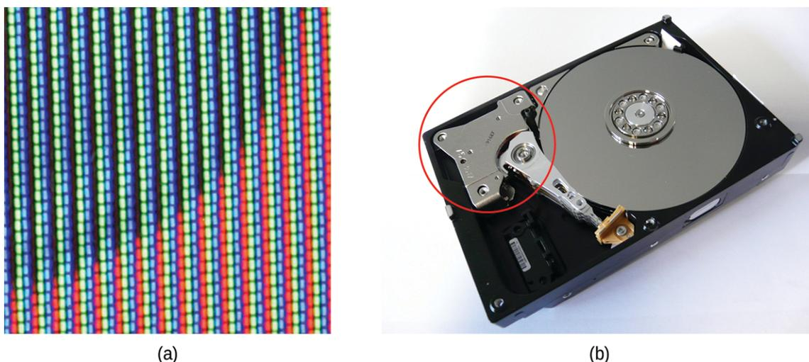
**FIGURE 19.3** (a) Europium is used in display screens for televisions, computer monitors, and cell phones. (b) Neodymium magnets are commonly found in computer hard drives. (credit b: modification of work by “KUERT Datenrettung”/Flickr)
