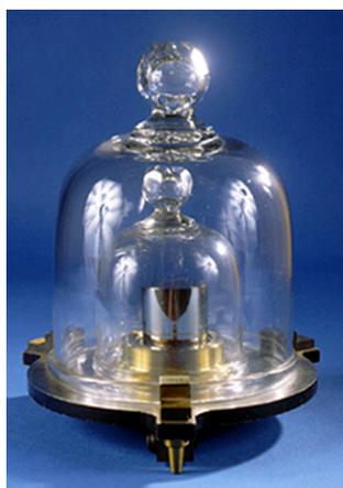
**FIGURE 1.24** This replica prototype kilogram as previously defined is housed at the National Institute of Standards and Technology (NIST) in Maryland. (credit: National Institutes of Standards and Technology)
