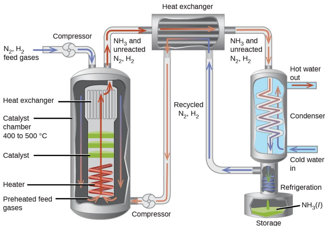
**FIGURE 13.9** The figure shows a typical industrial setup for the commercial production of ammonia by the Haber-Bosch process. The process operates under conditions that stress the chemical equilibrium to favor product formation.
