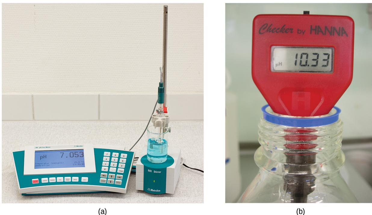
**FIGURE 14.4** (a) A research-grade pH meter used in a laboratory can have a resolution of 0.001 pH units, an accuracy of  $\pm 0.002$  pH units, and may cost in excess of \$1000. (b) A portable pH meter has lower resolution (0.01 pH units), lower accuracy ( $\pm 0.2$  pH units), and a far lower price tag. (credit b: modification of work by Jacopo Werther)
