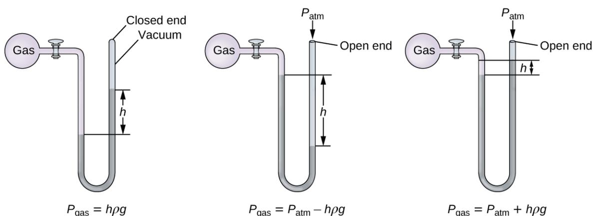
**FIGURE 9.5** A manometer can be used to measure the pressure of a gas. The (difference in) height between the liquid levels ( $h$ ) is a measure of the pressure. Mercury is usually used because of its large density.
