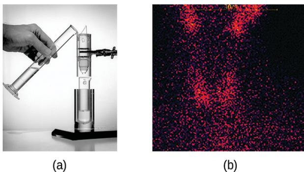
**FIGURE 21.25** (a) The first Tc-99m generator (circa 1958) is used to separate Tc-99 from Mo-99. The  $\text{MoO}_4^{2-}$  is retained by the matrix in the column, whereas the  $\text{TcO}_4^-$  passes through and is collected. (b) Tc-99 was used in this scan of the neck of a patient with Grave’s disease. The scan shows the location of high concentrations of Tc-99. (credit a: modification of work by the Department of Energy; credit b: modification of work by “MBq”/Wikimedia Commons)
