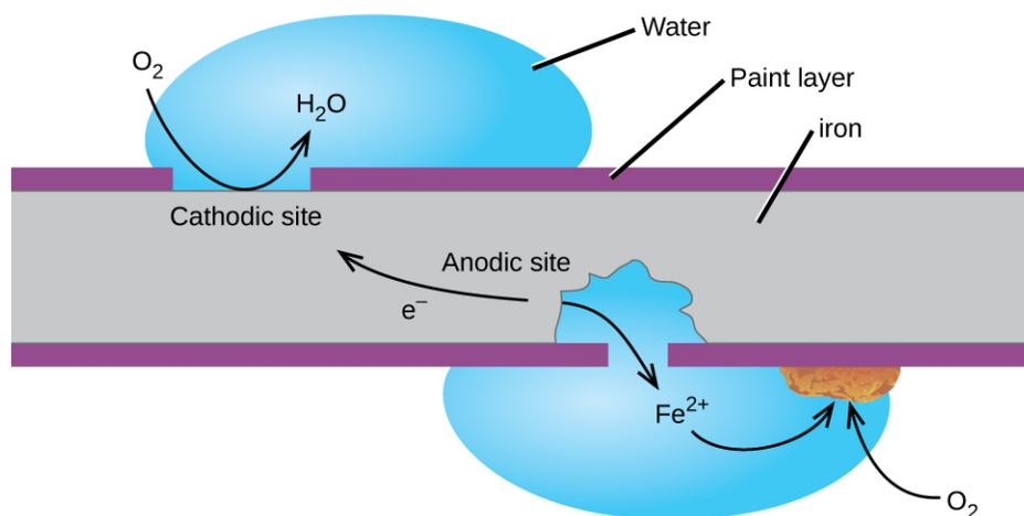
**FIGURE 17.16** Corrosion can occur when a painted iron or steel surface is exposed to the environment by a scratch through the paint. A galvanic cell results that may be approximated by the simplified cell schematic  $\text{Fe}(s) \mid \text{Fe}^{2+}(aq) \parallel \text{O}_2(aq), \text{H}_2\text{O}(l) \mid \text{Fe}(s)$ .
