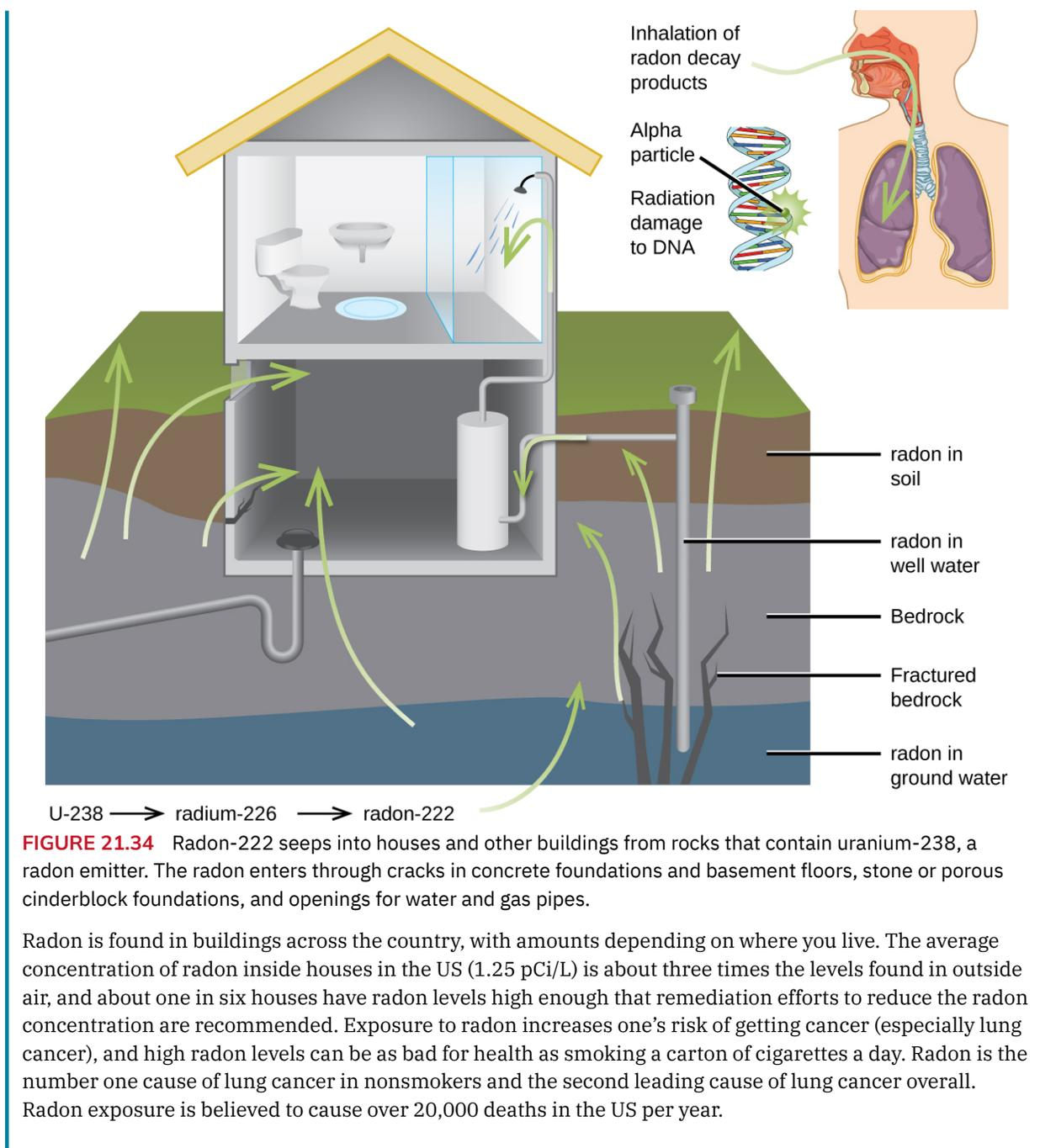
**FIGURE 21.34** Radon-222 seeps into houses and other buildings from rocks that contain uranium-238, a radon emitter. The radon enters through cracks in concrete foundations and basement floors, stone or porous cinderblock foundations, and openings for water and gas pipes.
