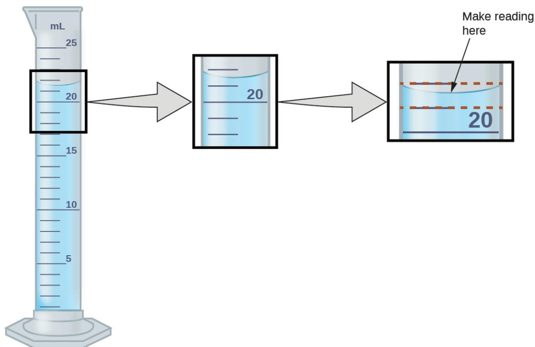
**FIGURE 1.26** To measure the volume of liquid in this graduated cylinder, you must mentally subdivide the distance between the 21 and 22 mL marks into tenths of a milliliter, and then make a reading (estimate) at the bottom of the meniscus.
