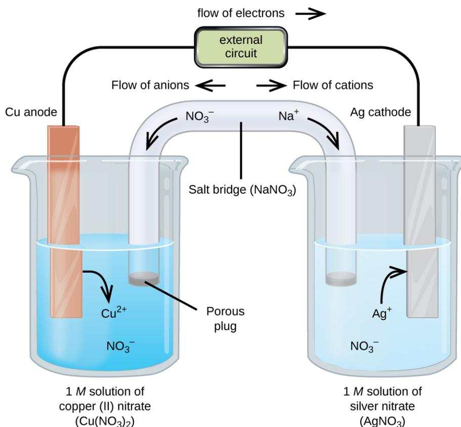
**FIGURE 17.3** A galvanic cell based on the spontaneous reaction between copper and silver(I) ions.
