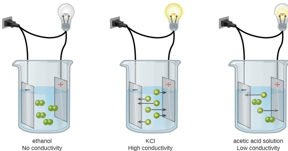
**FIGURE 11.6** Solutions of nonelectrolytes such as ethanol do not contain dissolved ions and cannot conduct electricity. Solutions of electrolytes contain ions that permit the passage of electricity. The conductivity of an electrolyte solution is related to the strength of the electrolyte.
