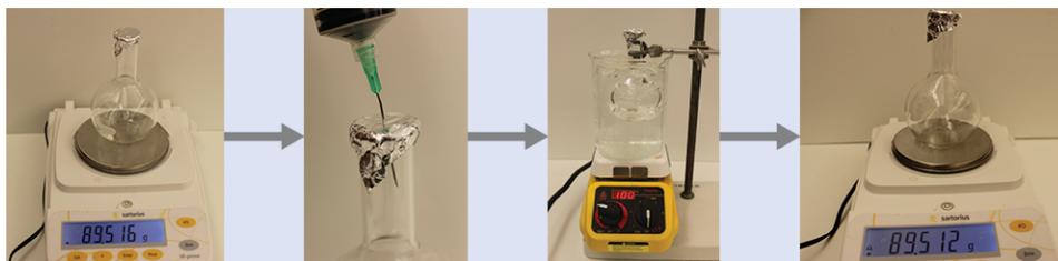
**FIGURE 9.19** When the volatile liquid in the flask is heated past its boiling point, it becomes gas and drives air out of the flask. At  $t_l \rightarrow g$ , the flask is filled with volatile liquid gas at the same pressure as the atmosphere. If the flask is then cooled to room temperature, the gas condenses and the mass of the gas that filled the flask, and is now liquid, can be measured. (credit: modification of work by Mark Ott)
