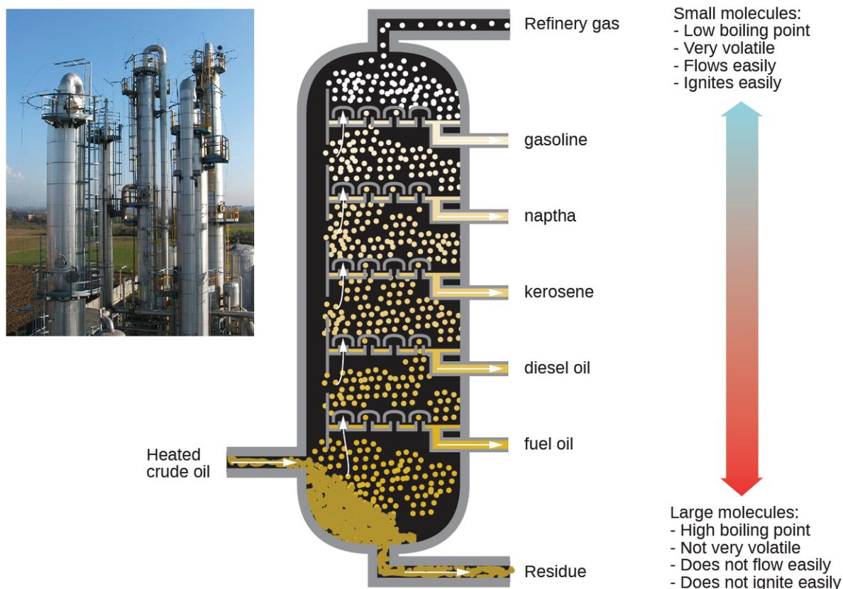
**FIGURE 20.6** In a column for the fractional distillation of crude oil, oil heated to about  $425\text{ }^\circ\text{C}$  in the furnace vaporizes when it enters the base of the tower. The vapors rise through bubble caps in a series of trays in the tower. As the vapors gradually cool, fractions of higher, then of lower, boiling points condense to liquids and are drawn off. (credit left: modification of work by Luigi Chiesa)
