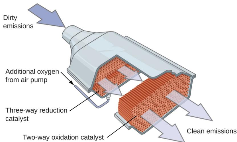
**FIGURE 12.24** A catalytic converter allows for the combustion of all carbon-containing compounds to carbon dioxide, while at the same time reducing the output of nitrogen oxide and other pollutants in emissions from gasoline-burning engines.
