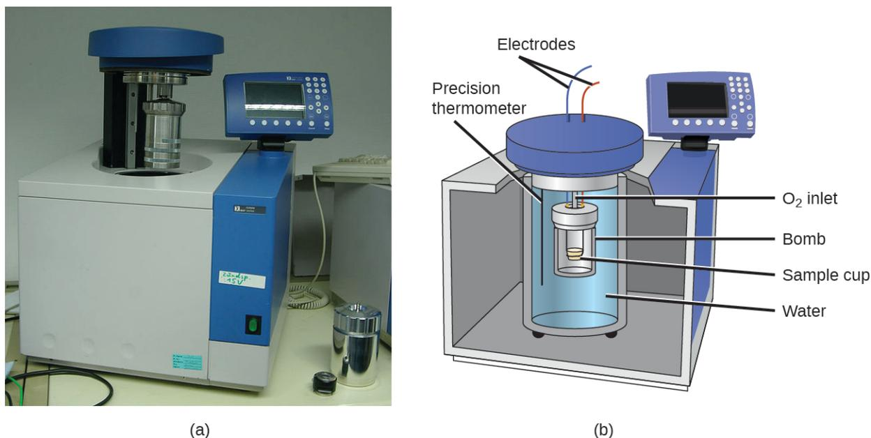
**FIGURE 5.17** (a) A bomb calorimeter is used to measure heat produced by reactions involving gaseous reactants or products, such as combustion. (b) The reactants are contained in the gas-tight “bomb,” which is submerged in water and surrounded by insulating materials. (credit a: modification of work by “Harbor1”/Wikimedia commons)
