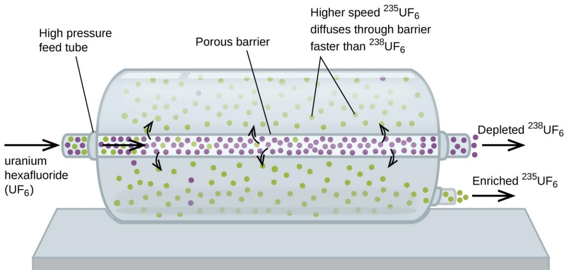
**FIGURE 9.30** In a diffuser, gaseous  $\text{UF}_6$  is pumped through a porous barrier, which partially separates  $^{235}\text{UF}_6$  from  $^{238}\text{UF}_6$ . The  $\text{UF}_6$  must pass through many large diffuser units to achieve sufficient enrichment in  $^{235}\text{U}$ .
