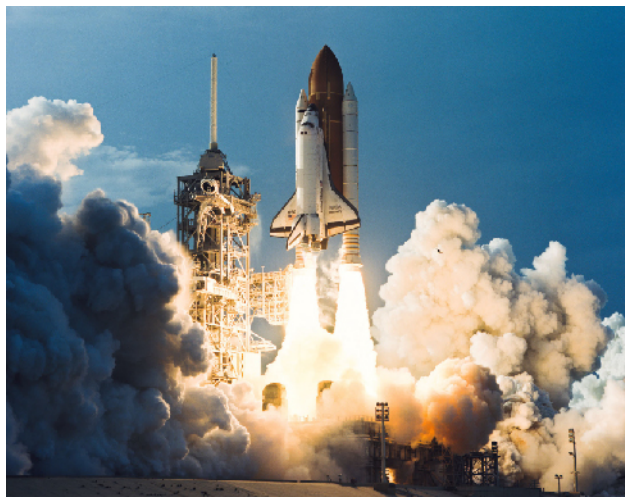
Figure 3.7 Demonstrating Newton’s Third Law. The U.S. Space Shuttle (here launching Discovery ), powered by three fuel engines burning liquid oxygen and liquid hydrogen, with two solid fuel boosters, demonstrates Newton’s third law. (credit: modification of work by NASA)
