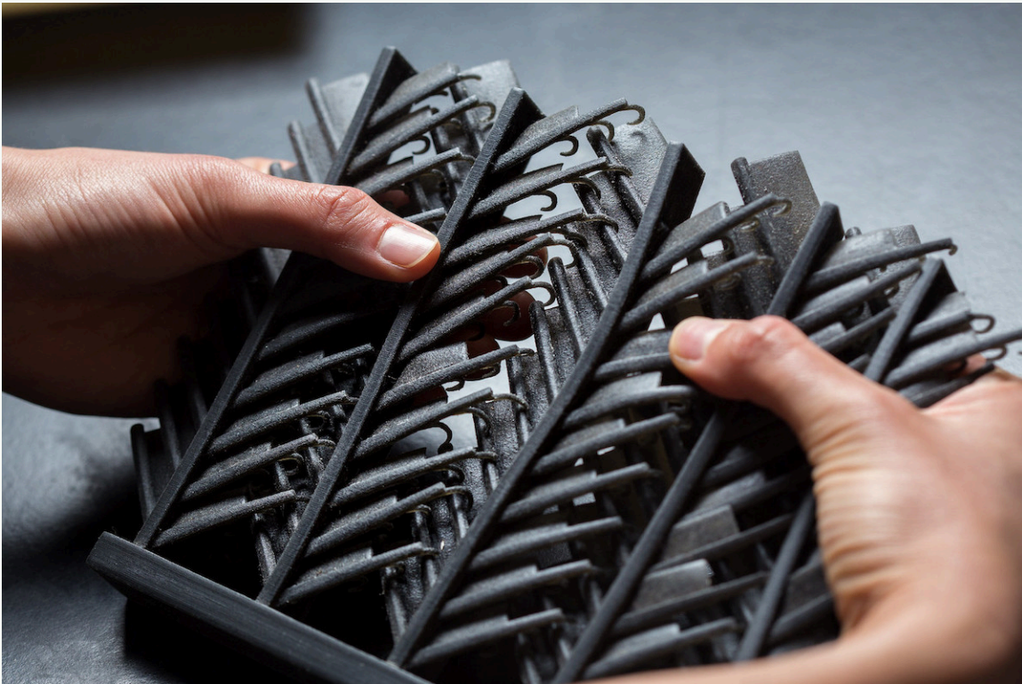
Figure 4.7 Biomimicry is exemplified in the creation of artificial feathers, initially at a much larger scale than actual feathers. This design includes most aspects of the feathers, including the hooks at the ends of the barbules, which in natural feathers are invisible without magnification. (credit: Modification of “20180322-MeyersLab-Feathers-3492-export-8MP” by UC San Diego School of Engineering/Flickr, CC BY 2.0)
