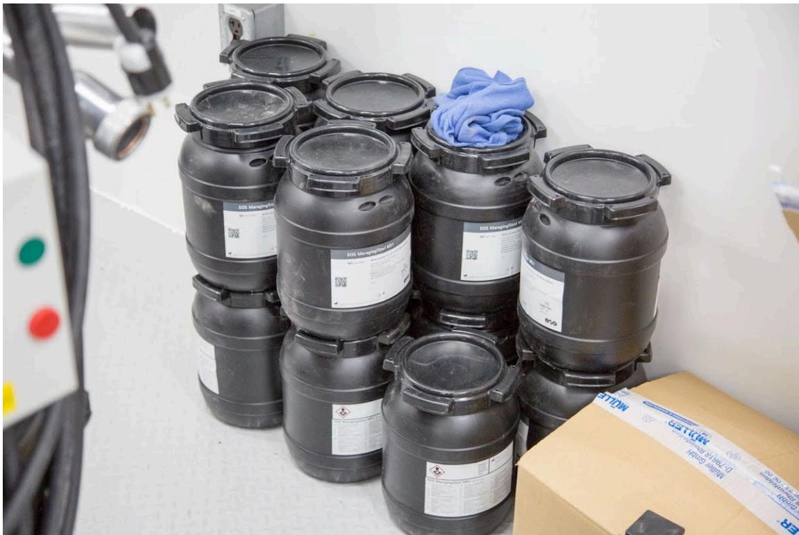
Figure 8.10 Each of these canisters contain 10 kilograms, about 22 pounds, of powdered steel, used in the construction process with the EOS M 400 3-D metal printer. Each container is valued at $7,000. The 3-D printer also used soft aluminum or titanium powder to construct hard to find parts or design and build tools specifically for a project at PPB, MDMC. (credit: Marine Corps photo by Keith Hayes on DVIDS, Public Domain)
