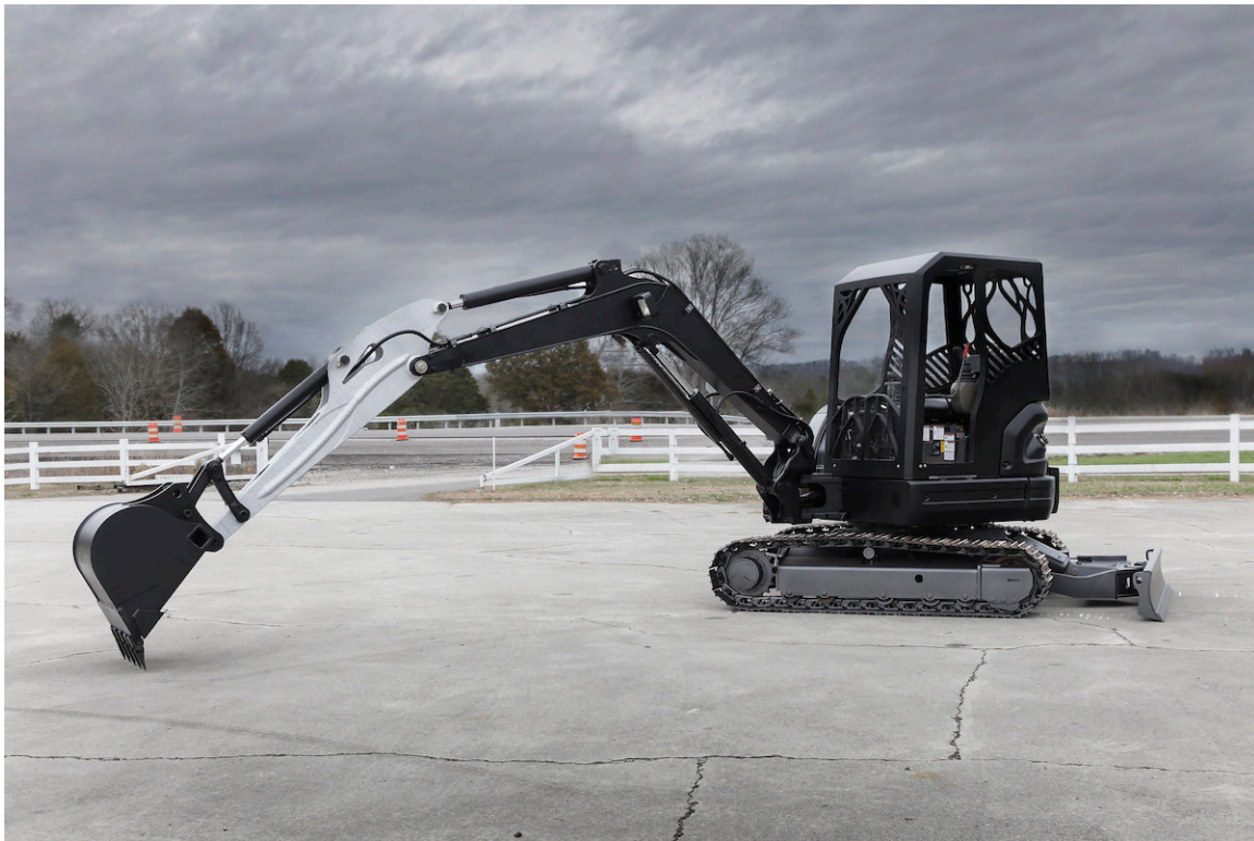
Figure 4.11 Large-scale DED excavator boom 3D printed at the U.S. Department of Energy's Manufacturing Demonstration Facility at Oak Ridge National Laboratory (credit: Modification of "Project AME" by Oak Ridge National Laboratory/Flickr CC BY 2.0)
