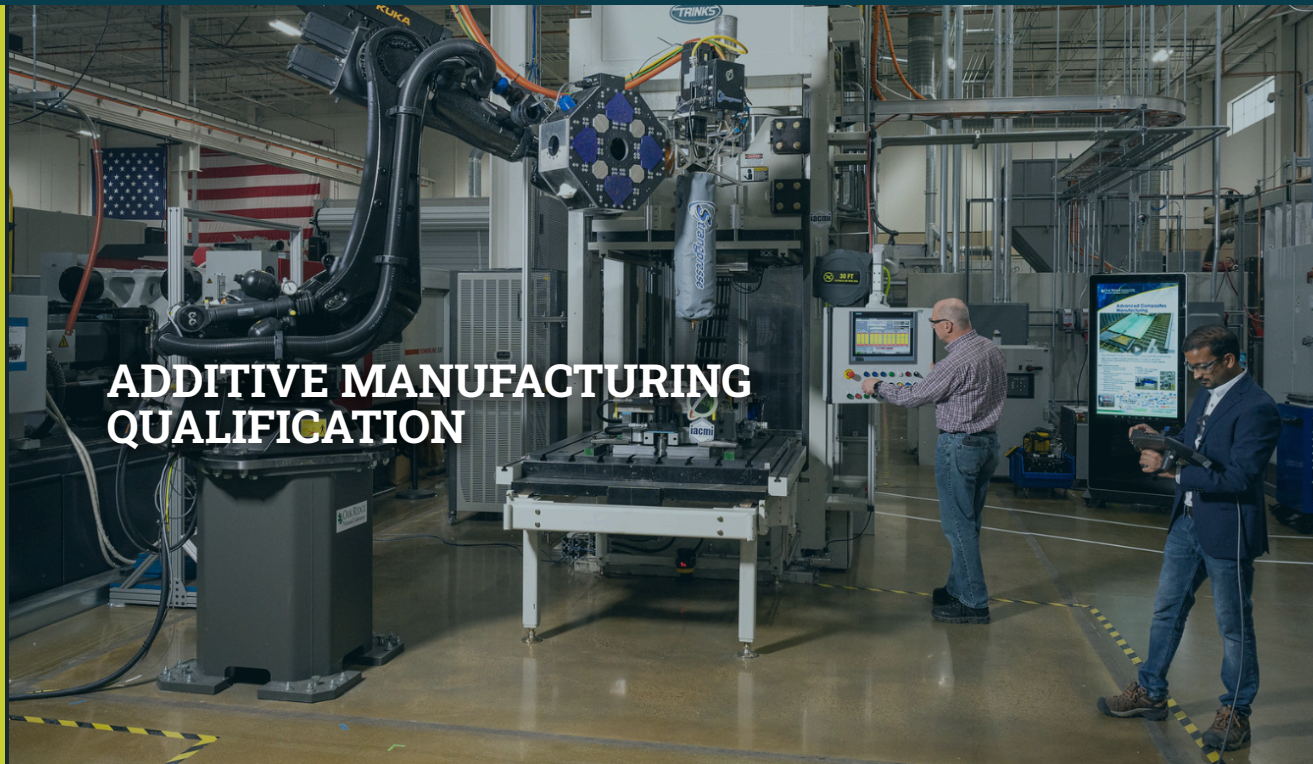
Figure 6.1 Qualification involves evaluating a manufacturer’s ability to undertake each step in the part or system creation process. This becomes even more complex when two or more processes are involved in the creation of a part. This hybrid additive manufacturing system combines 3D printing with compression molding. It is capable of producing parts made of one material as well as building multiple materials, such as interconnected metals and polymers. But before such builds are done at production scale and pace, the machine, the build processes, the personnel, and the testing approaches all must be evaluated and qualified as effective and up to standard. (credit: Modification of “Additive Manufacturing Compression Molding System” by Oak Ridge National Laboratory/Flickr, CC BY 2.0).
