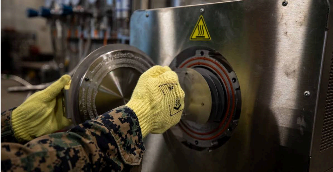
Figure 7.2 Operators and manufacturers may not consider post-processing steps, such as sintering as shown here, to have a significant digital component. However, some printers, processes, and end-users may require a detailed transcript of the precise conditions of sintering in order to undertake further steps. (credit: U.S. Marine Corps photo by Cpl. Jamin M. Powell on DVIDS, Public Domain)
