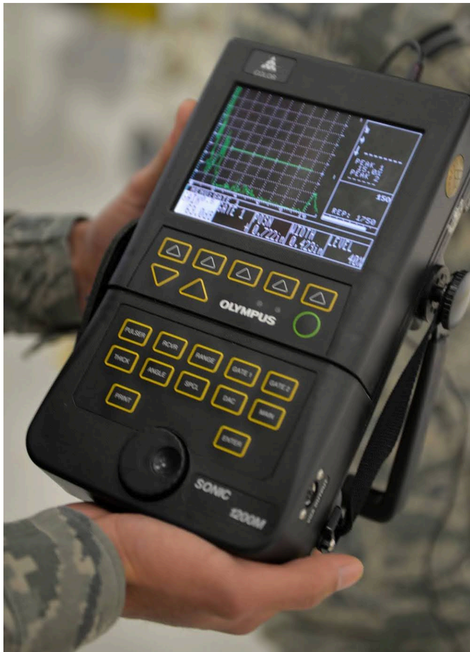
Figure 5.5 A non destructive inspection technician uses an ultrasonic flaw detector to analyze a damaged aircraft panel. (credit: U.S. Air Force photo/Senior Airman Andrea Posey on DVIDS, Public Domain)
