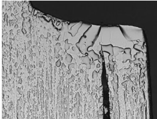
Figure 7.8 This highly magnified view of a weld reveals a gap in the form of the darker region to the right of the center. Quality assurance personnel (or software) would need to assess whether or not this gap constitutes a risk, and whether it requires repair or a complete rebuild. Ideally, that quality assurance data – including the size and location of the gap itself – would be captured in the digital thread. (credit: Modification of “Art of Science 2023” by Oak Ridge National Laboratory/Flickr, CC-BY 2.0)
