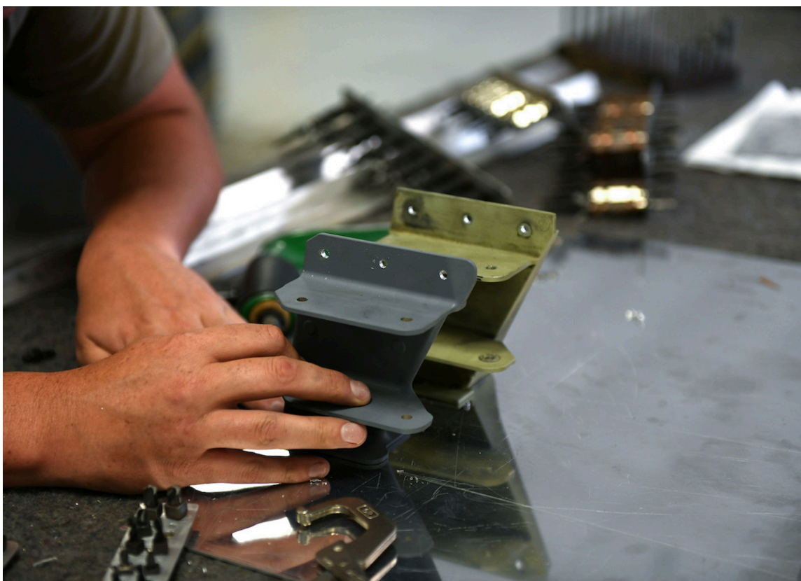
Figure 3.6 An Air Force technical specialist compares 3D printed pump bracket to the older bracket that needs replacement. The new part used a stronger alloy to decrease the amount of repairs that are needed over time. (credit: U.S. Air Force photo by Airman 1st Class Jayden Ford on DVIDS, Public Domain.)
