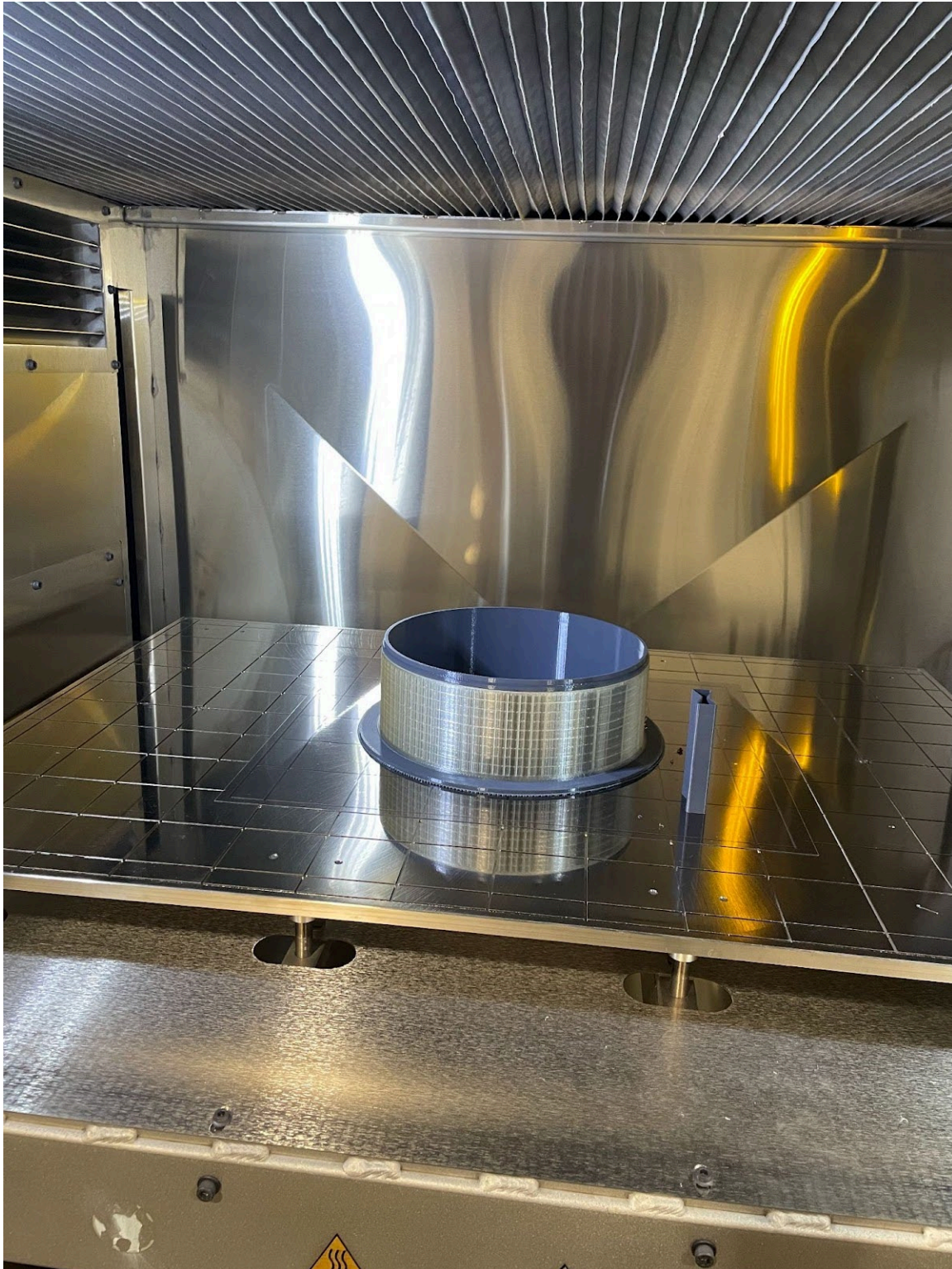
Figure 7.6 A Stratasys F900 3D printer manufactures a replacement part for an aircraft fuel mixing chamber on site at
